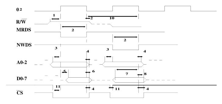
NB On the host side,  $0_2$  is the timing reference and R/W gives the direction of transfer. On the parasite side, the timing and direction are implied by MRDS or NWDS.
